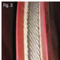
Fig. 3 Clear indentations of the rope profile
